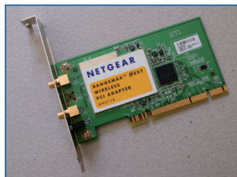
The WN311B is a PCI card that needs to be installed in your PC to give you full 802.11n speeds.
